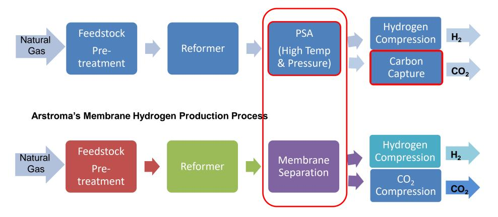
Arstroma's system does not require high temperature nor pressure. Less CAPEX and OPEX. → Lower Hydrogen Production Cost
