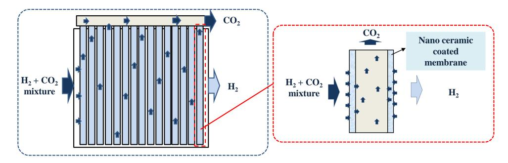
Not a hollow fiber type. Membrane in a sheet form.
